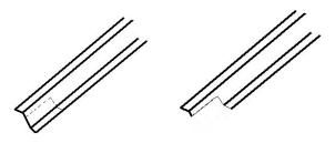
**6.** Apply a triangular bead of sealant to patio door. Remember to apply enough material to adhere both the frame and film.
