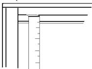
**5.** Using BondKap<sup>TM</sup> BK 2003, square cut the ends and cut a notch to fit over the existing BondKap<sup>TM</sup>.
